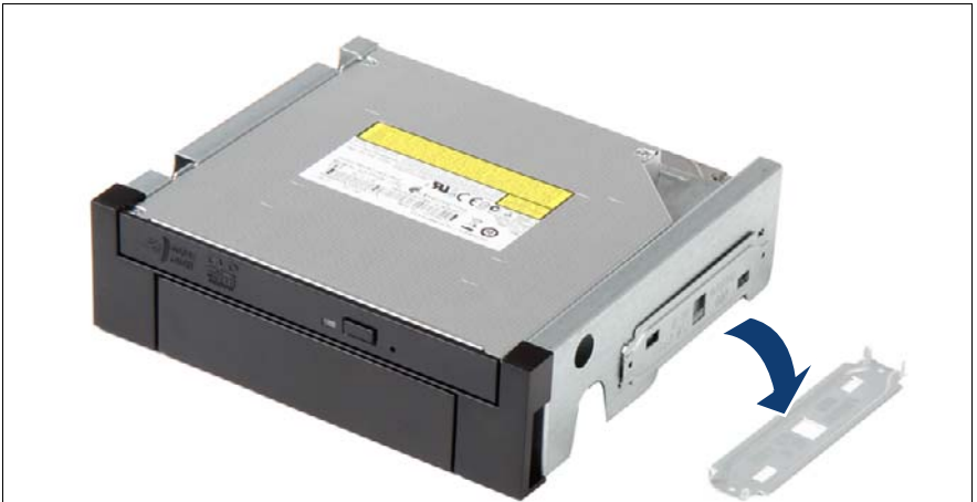
Figure 67: Removing the fixation plate of the 5.25-inch ODD/HDD bracket
